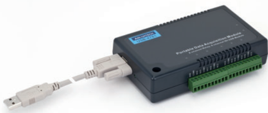
USB relay box (Art. No. 10450-1-0174) for processing various status messages of fans.
