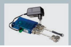
This interface converter permits bi-directional connection of RS232 devices (laptop or PDA) with bus-compatible devices (electronic commutation units with RS485 interface). The interface features electrical isolation between the RS232 and RS485 sides.
